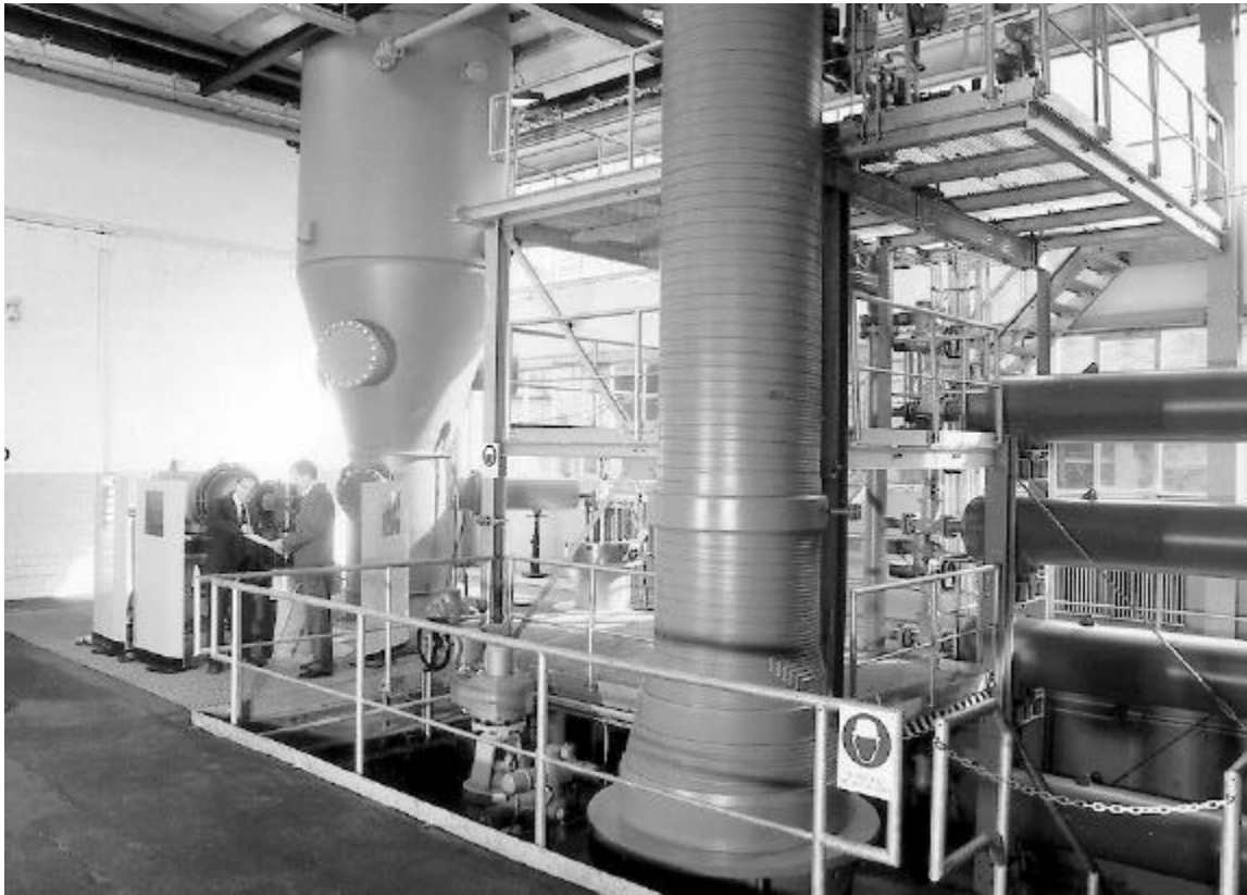
Figure 2: Bopp & Reuther large-scale test facility for pressure values up to 320 bar and a total volume of 20 m 3
